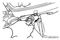
3. Place the tilt lock lever (if equipped) in the release/up position.
